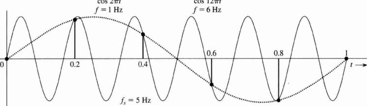
• In general, if a sinusoid of frequency f Hz is sampled at fs samples/sec, then sampled version would appear as samples of a continuous-time sinusoid of frequency  $|f_a|$  in the band 0 to fs/2, where:
