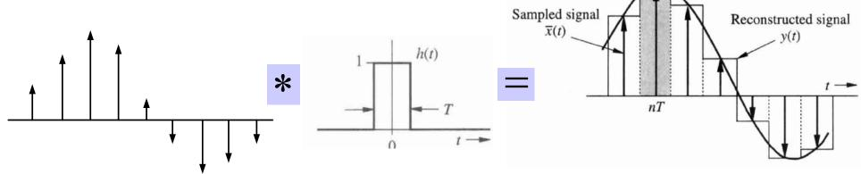
The effect of zero-order hold of the D/A converter is a non-ideal lowpass filter.
