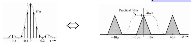
Sampling below Nyquist rate at 5Hz corrupts the signal.
