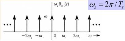
Therefore the sampled signal has a spectrum (convolution):
